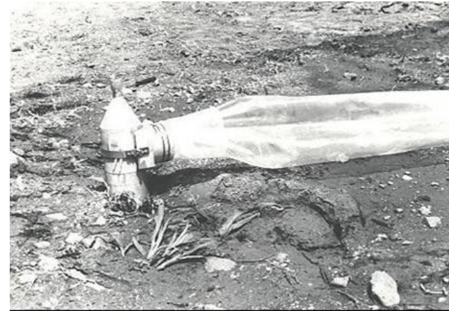
Fig.2a. Use of flexible distribution pipeline \Phi 200 , attached to a movable riser \Phi 150 mm for delivering water to a furrow set (15-30dka), ASSI, Chernogorovo.
